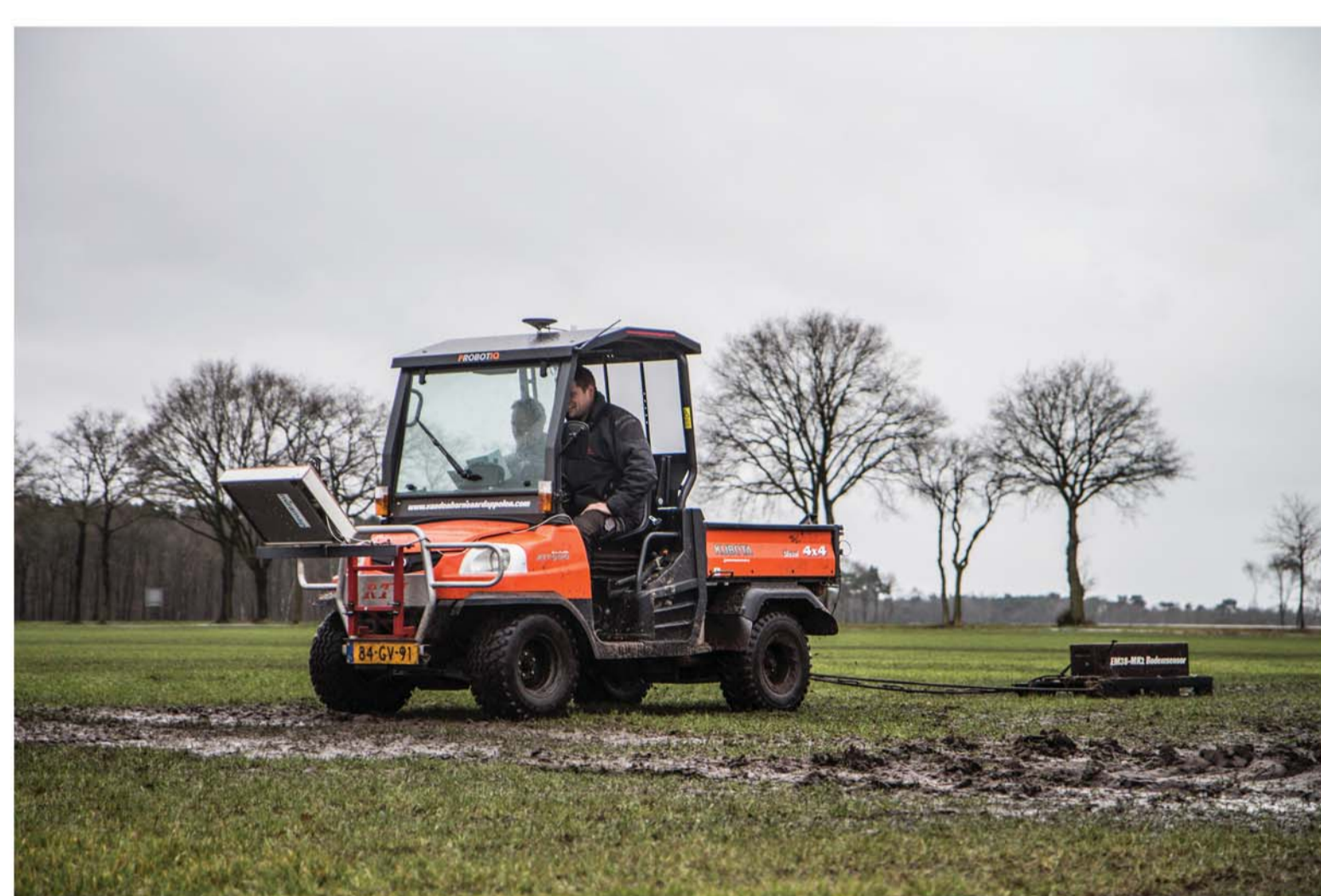
Figure 3: Kubota equipped in front with the mobile passive radiometer developed by Miramap and pulling the EM 38 over a bare soiled field
