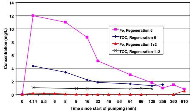
Figure 6. Quality of water pumped out during regenerations 1 and 2 (injection phase) and 6 (after storage phase).
