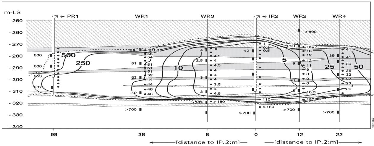
Figure 2. Spatial distribution of the infiltrate in the target aquifer after 826 days of injection (on October 13, 1998), with isochrones (in days) and indication of the observed travel time to the observation points.
