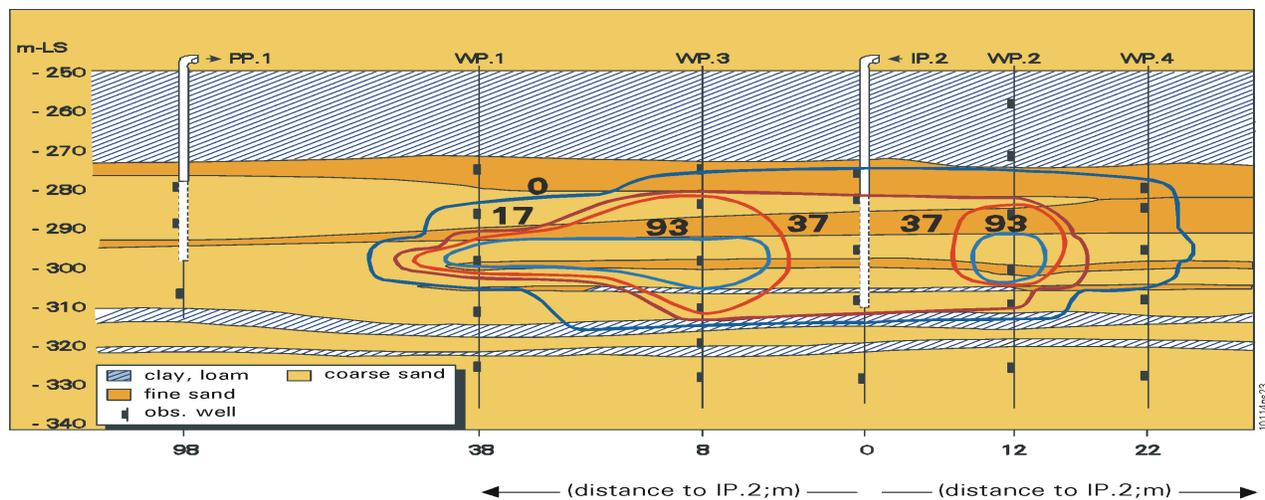
Figure 4. Shrinkage of the (sub)oxic zone in the target aquifer during stand still (storage), directly after 938 days of continuous injection of oxic surface water. Isolines indicate position of  $NO_3^-$  front 0, 17, 37, 93 days after injection stopped.
