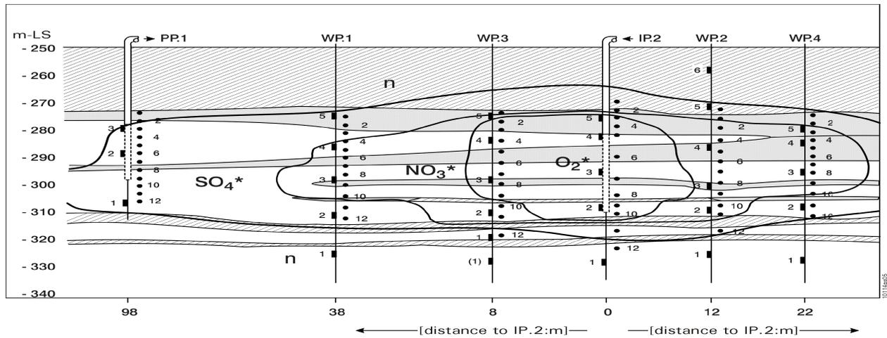
Figure 3. Redox zoning of the canal water injected into the Miocene sand aquifer, in October 1998 after 2.3 years of practically undisturbed recharge operation.  $O_2^*$  = containing oxygen (decreasing from 10 to 0 mg/L with distance from the injection well) and nitrate;  $NO_3^*$  = containing nitrate (decreasing from ca. 20 to 0 mg/L with distance);  $SO_4^*$  = containing sulphate (higher concentration than in input, due to pyrite oxidation); n = native groundwater.
