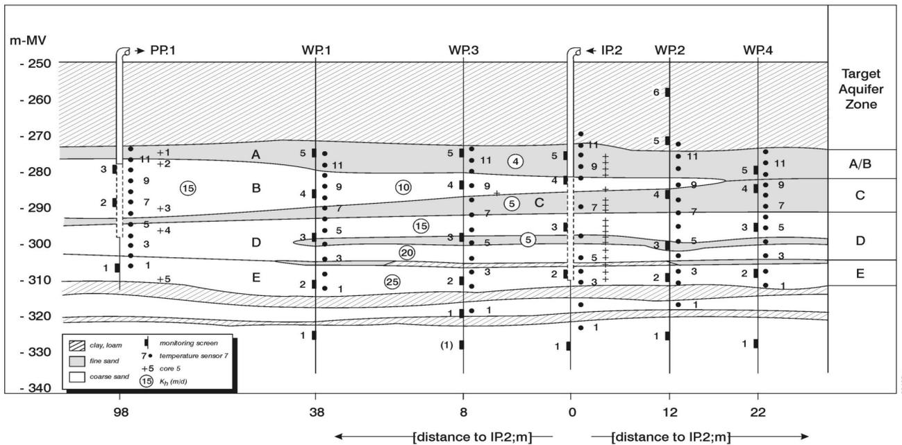
Figure 1. Position of the injection well (IP.2), monitoring wells (WP.1-4) and recovery well (PP.1) in cross section, showing well screens, temperature sensors, stratification of target aquifer, permeability distribution ( $K_h$  in m/d) and aquifer cores.
