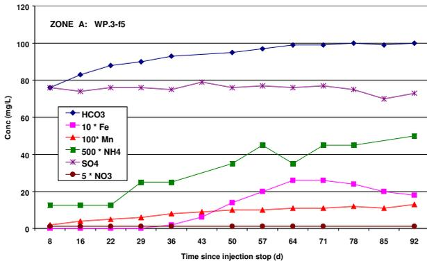
Figure 5. Quality changes in the injected bubble in zone A at 8 m from the injection well during stand-still (storage).
